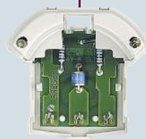
Overvoltage protection modules
